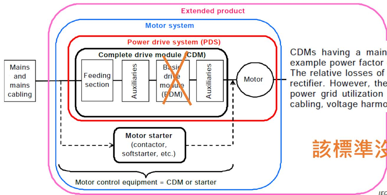
CDMs having a mains current THC of 10 % or lower (according to IEC 61000-3-12), for example power factor correction (PFC) fed CDMs, can be excluded from the IE classification. The relative losses of an active rectifier are typically twice the losses of a CDM with a diode rectifier. However, the efficiency contribution of an active rectifier can be seen in improved power grid utilization and lower system level losses and disturbances (power transformer, cabling, voltage harmonics, flicker).
